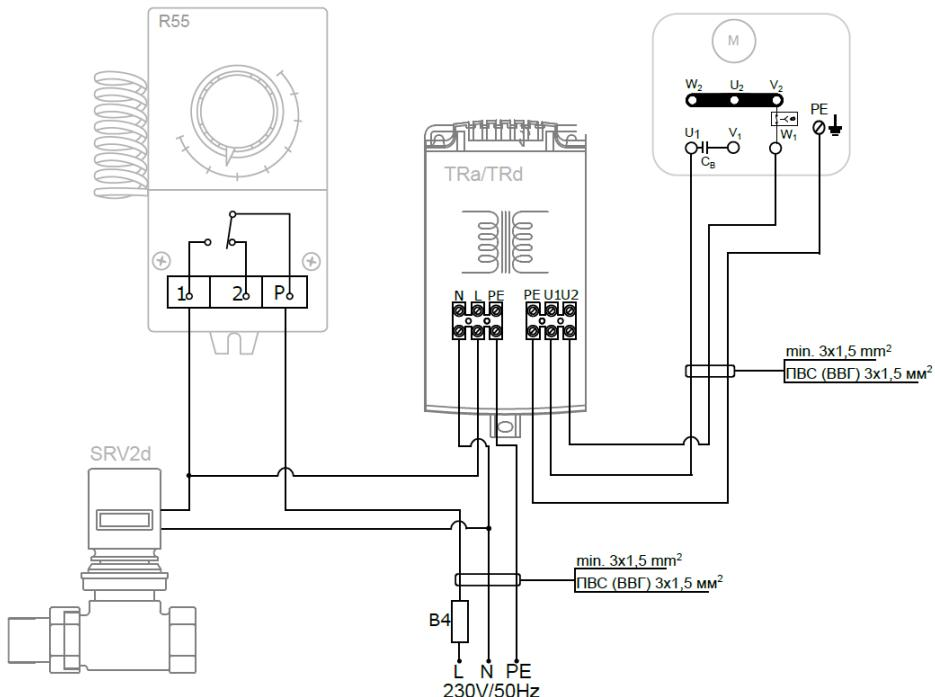
Thermostat R55 controls the operation of valve and TRa/TRd speed regulator. TRa/TRd allows for 5-step fan air flow switch. Wires size and type should be chosen by the designer.
