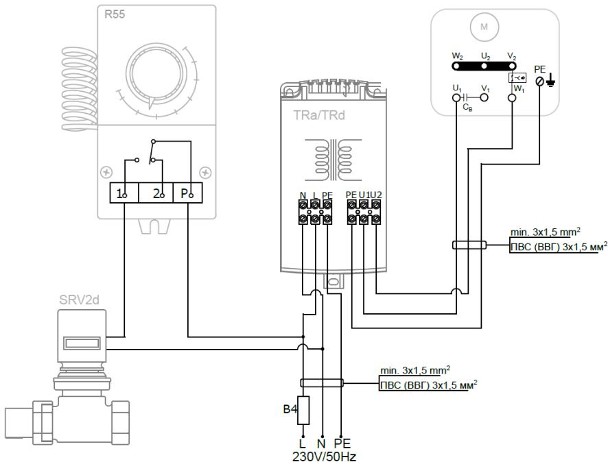
Thermostat R55 controls the operation of valve. TRa/TRd speed regulator allows for 5-step fan air flow switch. Wires size and type should be chosen by the designer.
